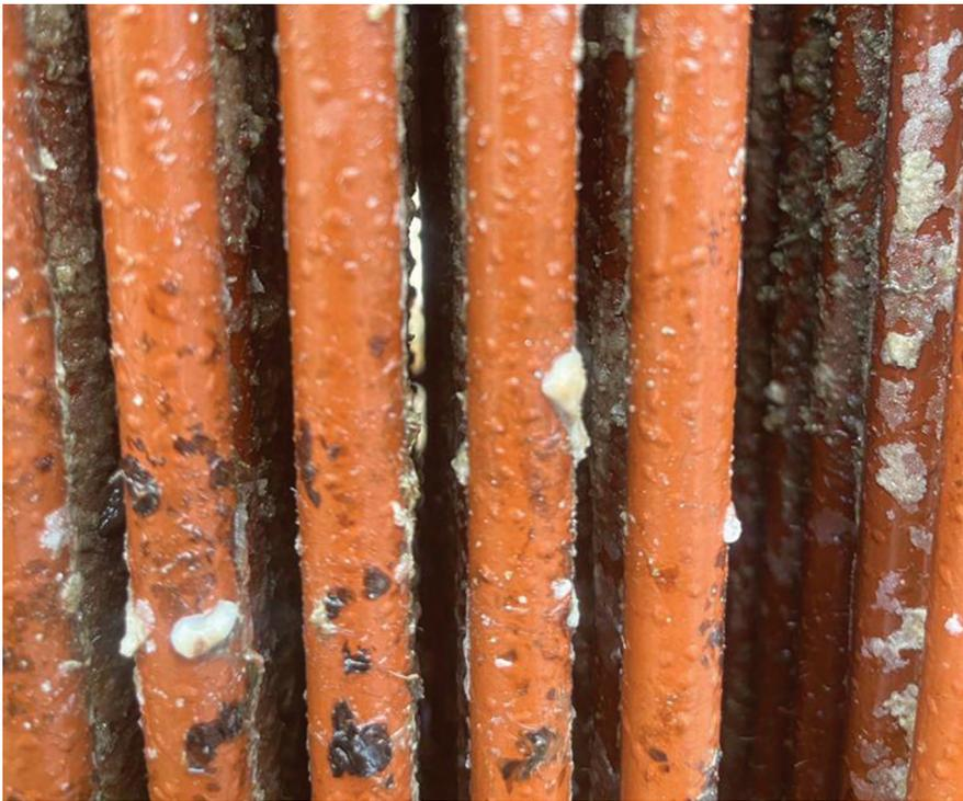
➤ A box cooler coated with baked phenolics after being in service for 5 years. The marine growth has been removed by cleaning and pressure washing. The condition of the coating requires a full re-coating.
