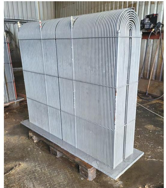
➤ A box cooler coated with Säkatonit Extra AR-F after 5 years in service. The cooler has only been pressure washed to remove marine growth. The smooth surface of the coating eases the removal of barnacles and other organic growth.
