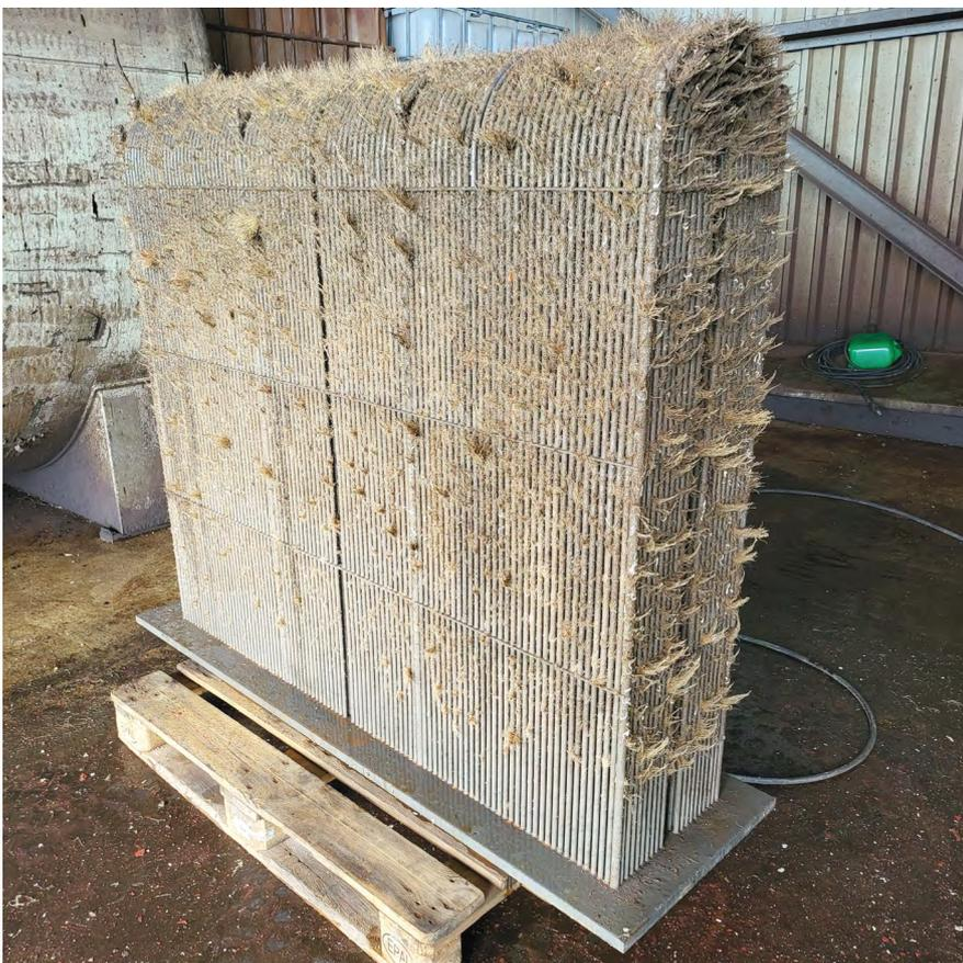
➤ A box cooler coated with Säkatonit Extra AR-F after 5 years in service, prior to pressure washing. The vessel operated in cooler water which can be derived from the amount of marine growth.
