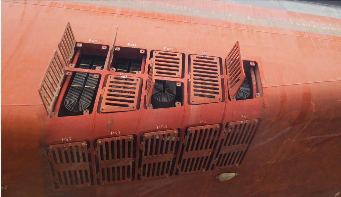
➤ A set of Box Cooler manufactured by Nederlandse Radiateurs Fabriek (NRF) installed in the aft portside sea chest of a vessel.
